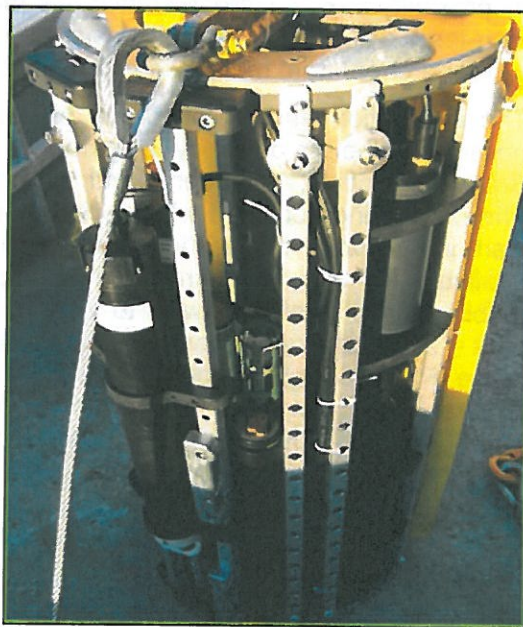
LOBO frame with representative sensors, data logger, and battery pack. (http://fau-hboi.loboviz.com/about/)
