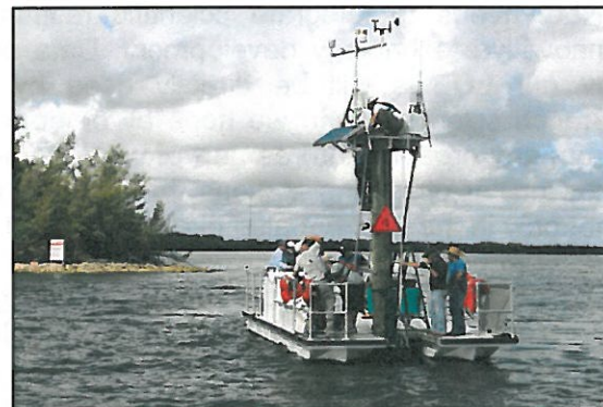
The Link Port LOBO site also has a weather station which allows direct linkage of local weather with water quality data.
