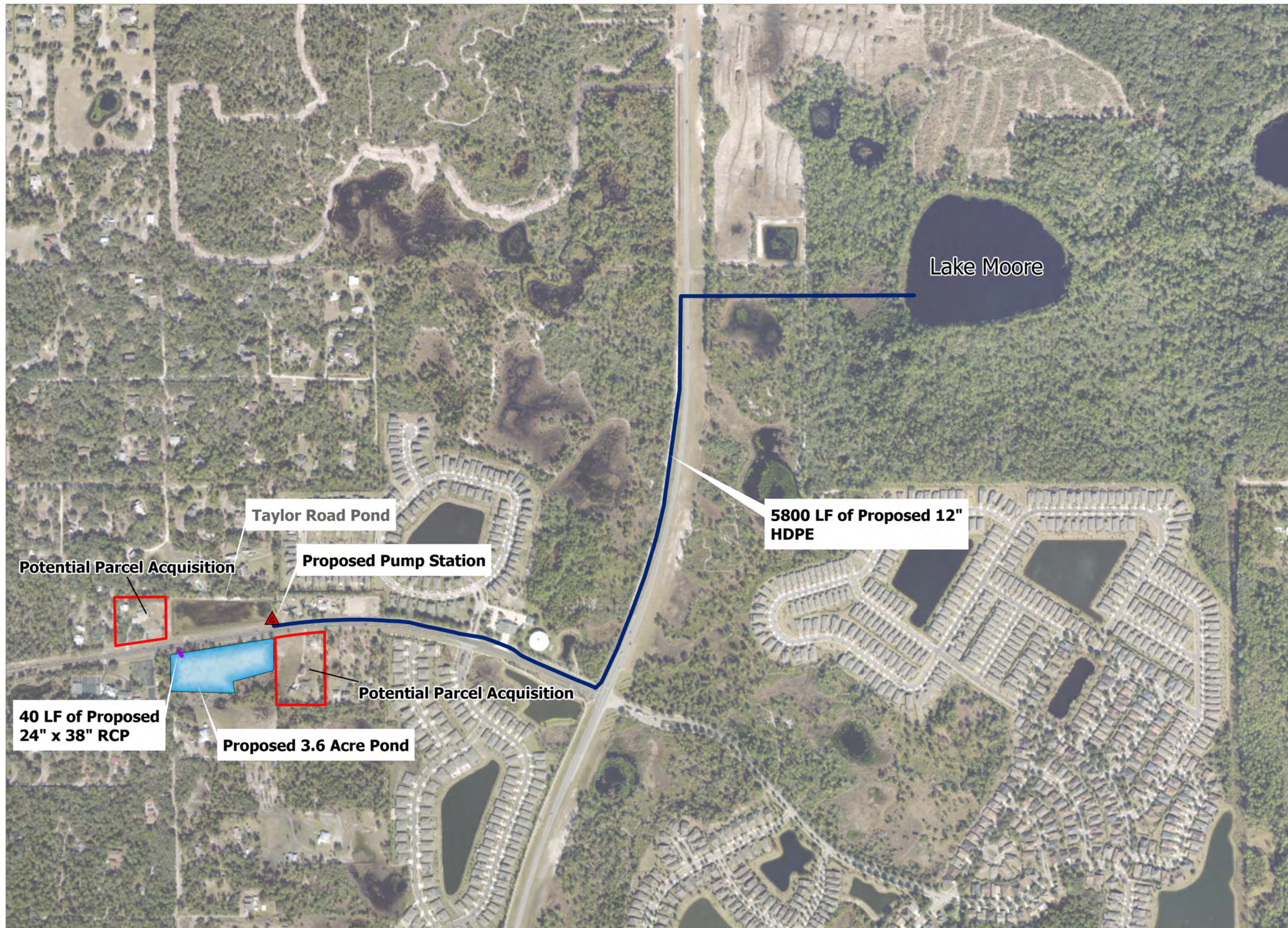
Figure 10 Alternative 2: Pump & Pond Taylor Road Stormwater Improvements
