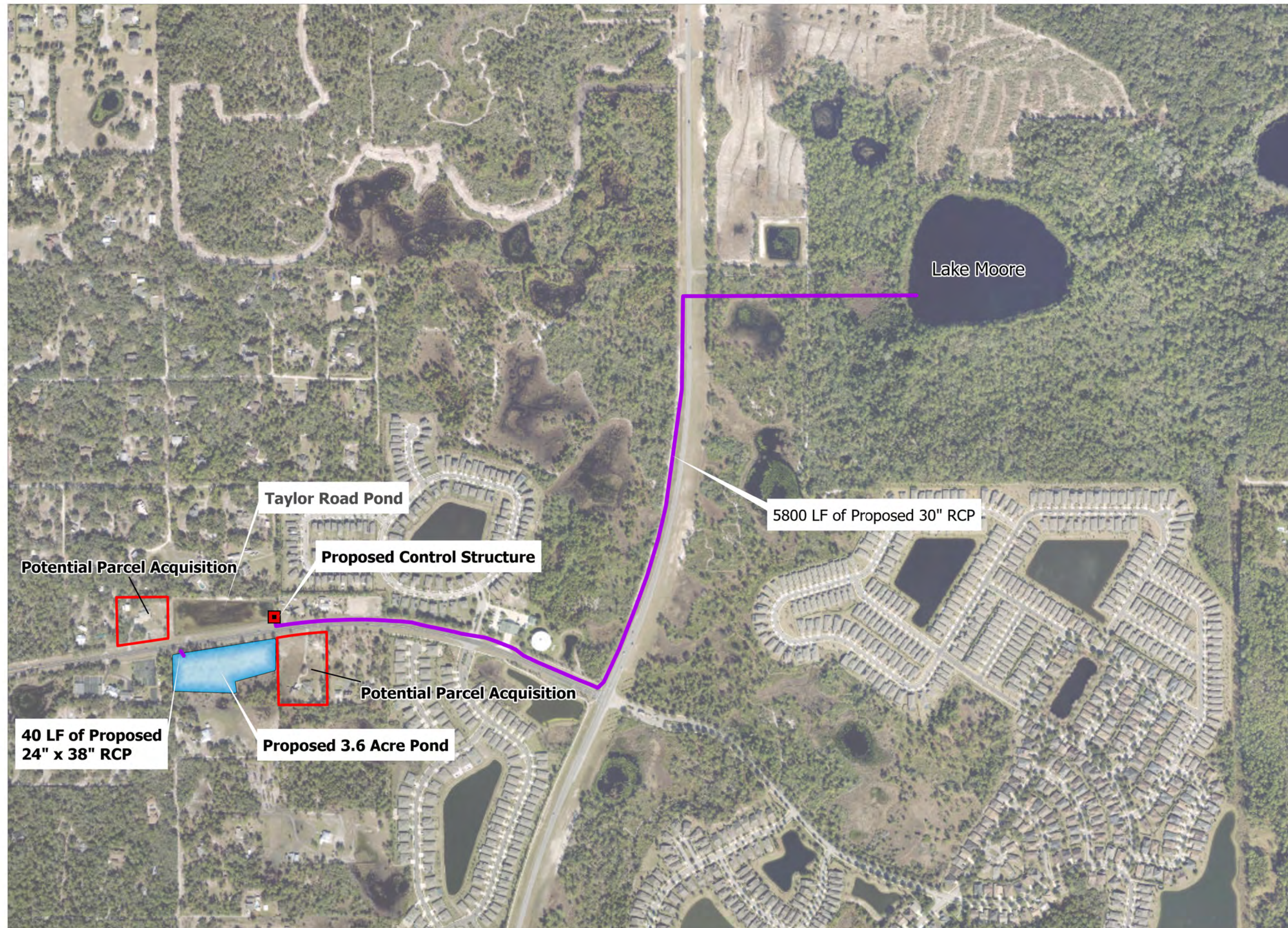
Figure 11 Alternative 3: CS & Pond Taylor Road Stormwater Improvements
