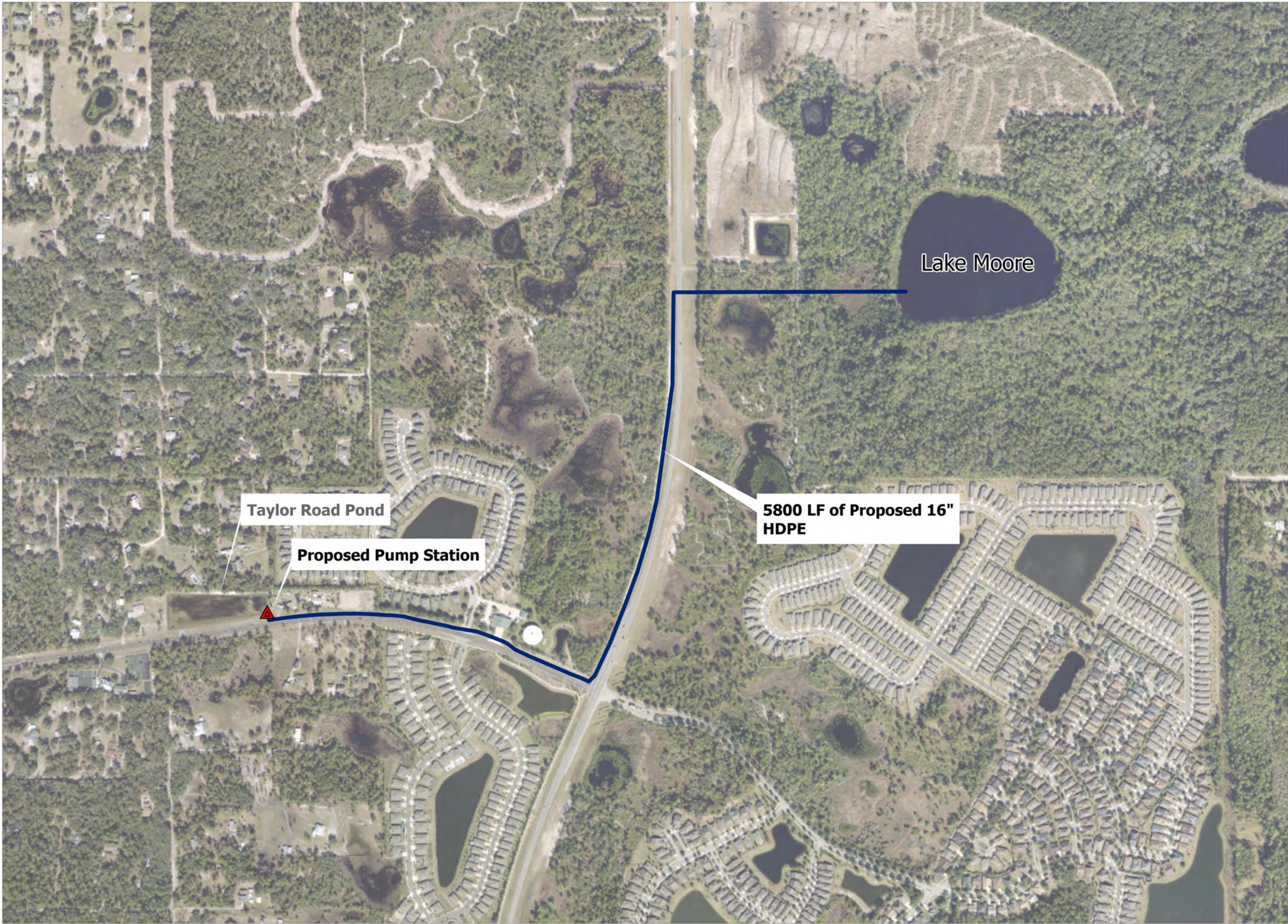
Figure 9 Alternative 1: Pump Only Taylor Road Stormwater Improvements
