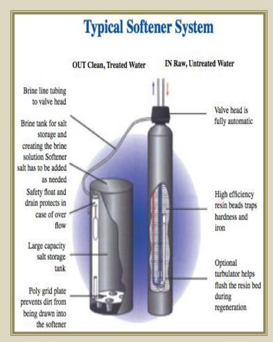
Water softeners operate on a simple principle: Calcium and magnesium ions in the water switch places with more desirable ions, usually sodium. The exchange eliminates two of the problems of hard water because sodium doesn't precipitate out in pipes or react badly with soap.
