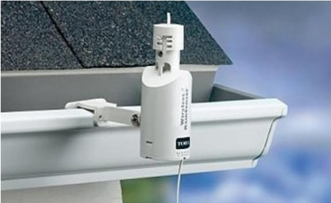
A rain sensor overrides the cycle of an automatic irrigation system when adequate rainfall has been received. The device is mounted outdoors, typically on the eave of a roof, and wired to the irrigation system's controller.
