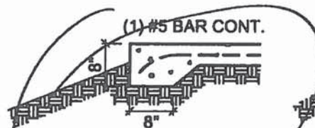
TYPE II MODERATE SLOPE FOOTING 2" / 12" - 1'-10"
