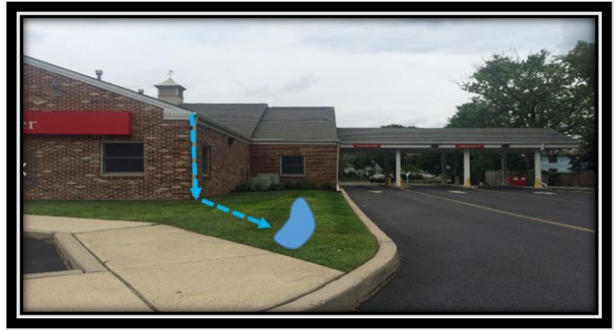
Figure 44: The image above depicts an example of disconnected impervious areas
