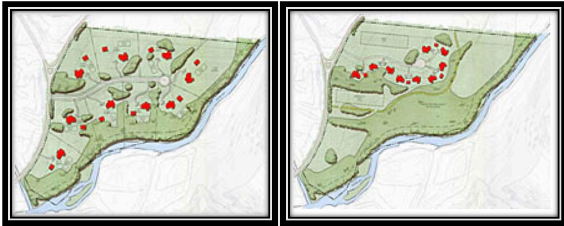
Figure 19: The left image displays a traditional development, and the right image displays a conservation development
